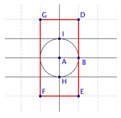
Adjust the radius of your compass to 2. With I as centre mark two points to the left and right of I. Then with H as centre mark two points to the left and right of H.
